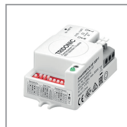
SmartSWITCH HF 5DPf For automatic on/off switching of luminaires with electronic ballasts and LED drivers. Bright-out function: luminaire is not switched on if there is adequate brightness. Delay time, detection range and light value for the bright-out function can be set via 9 dip switches.
