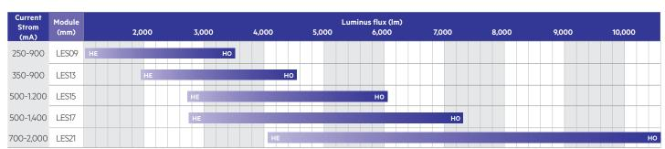
Operating mode; high efficiency (HE) to high output (HO) @  $3.000\,\mathrm{K}$ ; CRI > 80; tp  $65\,^{\circ}\mathrm{C}$
