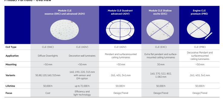
Module CLE provides perfectly homogeneous illumination in round and square luminaires with no shadow effects. As an efficient, high-quality and user-friendly system solution, CLE is the ideal replacement for ring-shaped and TC DD fluorescent lamps.
