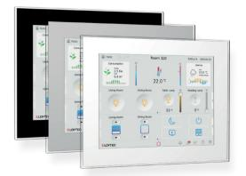
Frameless glass front and capacitive touch (also available with Anodized aluminum front frame)
