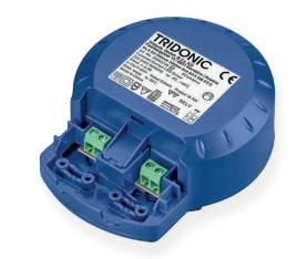
Dimensions Output Max. input Max. output current voltage power Ø75x95x41.3mm 255 mA 10.5 W 50 V 50 V Ø88x106,5x41,5mm 530 mA 21.3 W
